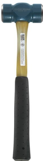
Klein Tools Lineman's Double-Face Hammer is designed for pole-line work. It is rugged and well-balanced, with the weight to drive lag bolts. The forged, tempered-steel head is only 3-3/4-Inch (95 mm) long for use in tight areas.
